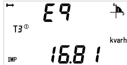
Current forward reactive total energy
